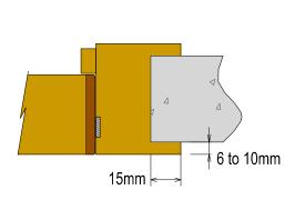
6-10mm is the maximum a frame is permitted to be proud of the structural surround when combined with a 15mm bolection return. Projecting frames outside these dimensions will require specific test evidence or assessment.
