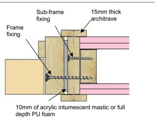
Guidance for various methods of sealing the frame to structural opening gap is also given in BS 8214: 2016, "*Timber*—based fire door assemblies. Code of Practice", which may be referred to where appropriate.
