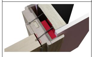
Split frames are permitted providing that both frame sections are secured to the wall in accordance with section 11.5. Furthermore, the main frame section (from which the door is hung) must be constructed to at least the minimum door frame section size (width and depth) as per the requirements noted in this report — see door frame section. The extension piece must be constructed using the same timber species as the main frame section.
