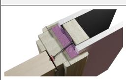
Instances where the door frame and the wall of the same depth such that architraves are fitted flush to both faces. Note that the minimum door frame section size (width and depth) must be as per the requirements noted in this report – see door frame section.
