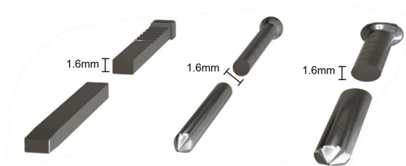
Figure 6.2 – Round, Oval & Rectangular pin detail – minimum dimension 1.6mm
