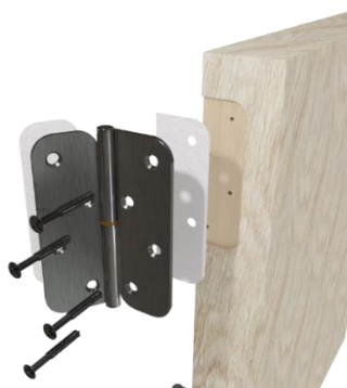
Example of hinge protection detail
