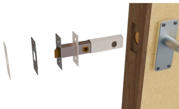
Example of lock & latch protection detail
