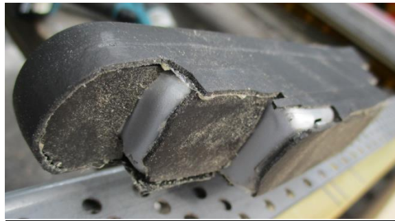
Image showing intumescent protection applied to the hinge body (leaf blade only)
