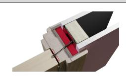
Instances where the door frame and the wall of the same depth such that architraves are fitted flush to both faces. Note that the minimum door frame section size (width and depth) must be as per the requirements noted in this report – see door frame section.
