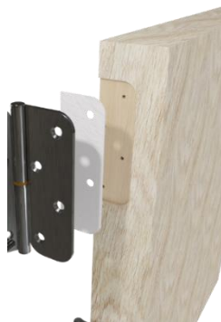
Example of hinge protection detail
