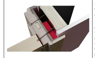
Split frames are permitted providing that both frame sections are secured to the wall in accordance with section 11.5.
