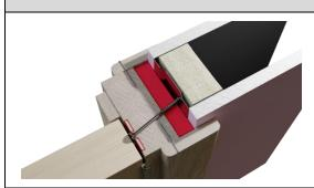
Instances where the door frame and the wall of the same depth such that architraves may be fitted flush to both faces.
